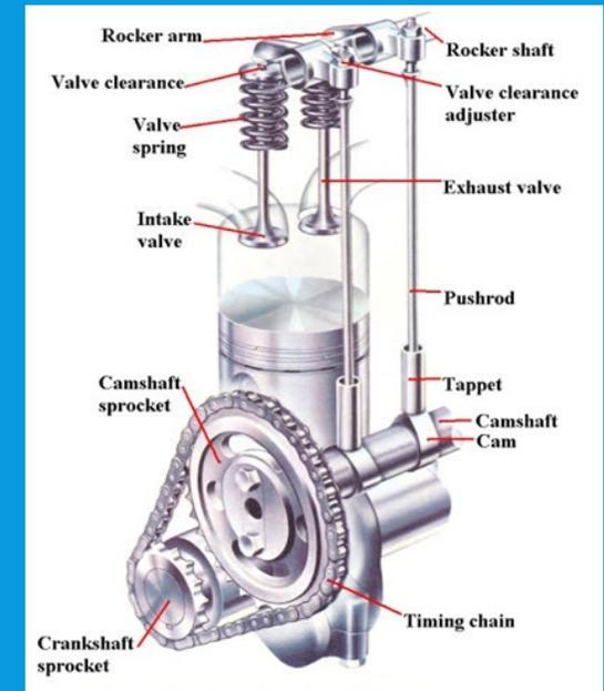
The valve mechanism is operated by a camshaft, which is driven by a gear that mates with another gear attached to the crankshaft. The camshaft rotates at one-half the speed of the crankshaft.
