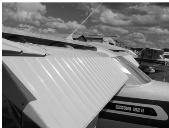
Ensure flaps do not retract if pushed, flap rollers allow small amount of play in down position.
