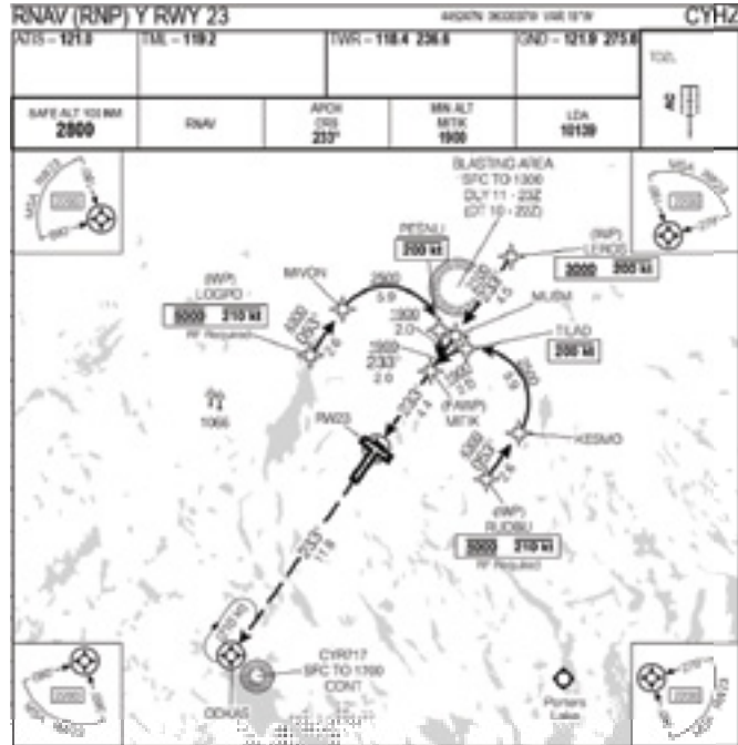
Figure 9.6 – CYHZ RNAV (RNP) Y RWY 23 with Left and Right “RF REQUIRED” IWP to FAWP Transitions
