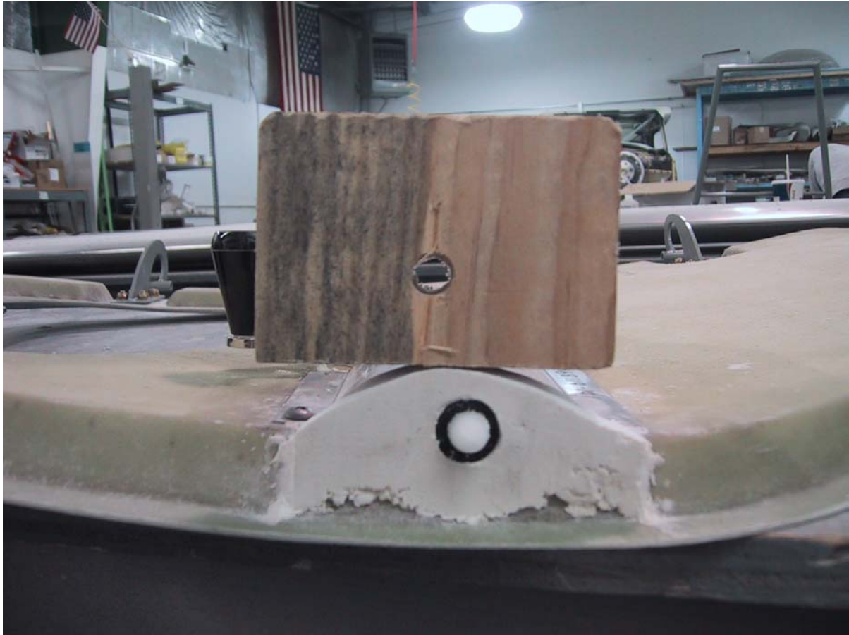
Figure H: Method of damming the structural pour for the baggage door latch pin.
