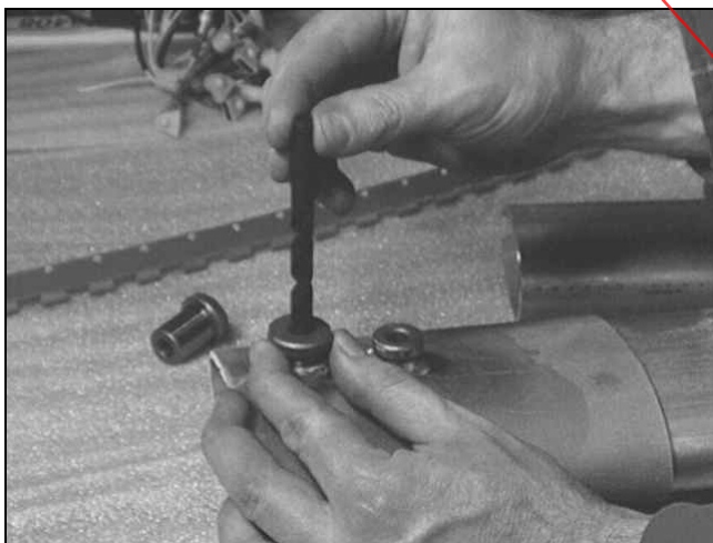
Figure 72: Marking the Hole Center
