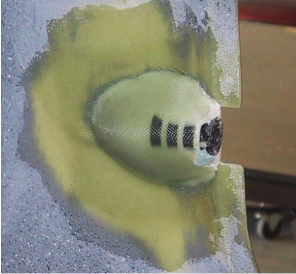
Figure 139.2: Baggage Door Latch Pin Receiver Sleeve Installation
