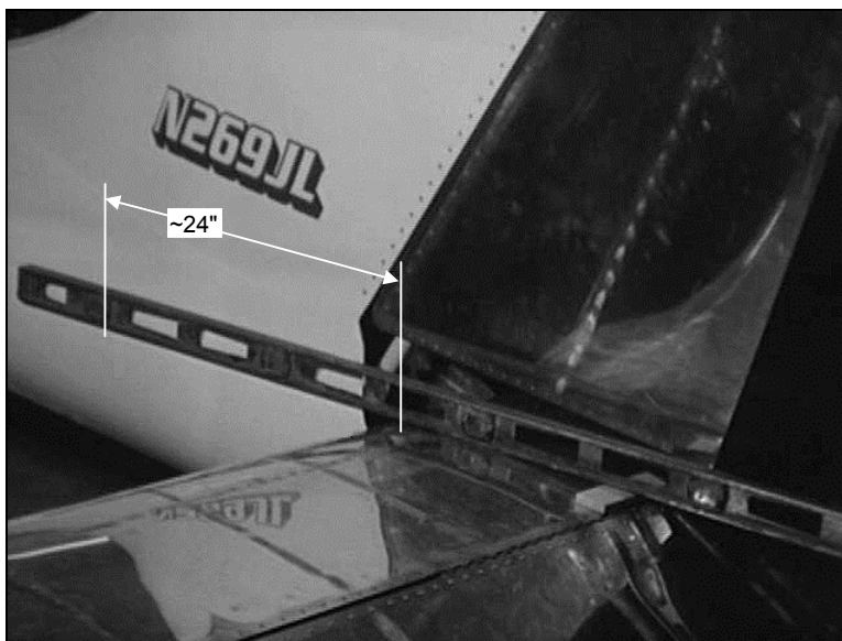
Figure 35: Marking the Stabilizer Chord Reference Lines
