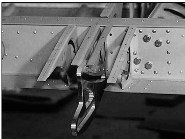
Figure 68: Flap Track Installation
