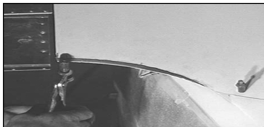
Figure 150: Clamping the Hatch Trailing Edge
