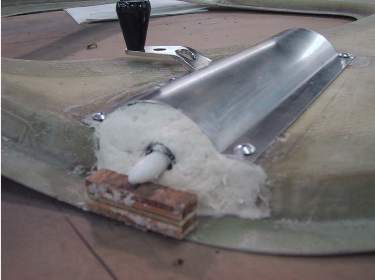
Figure 138.6: Position of the Sleeve and Pin Relative to the Foam Core Recess.
