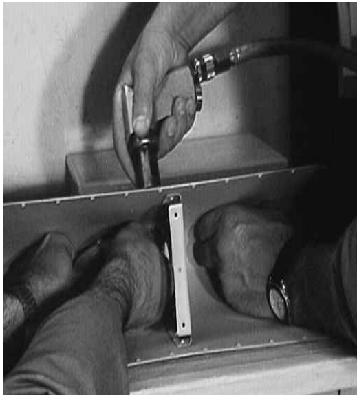
Figure 81: Riveting the Leading Edge
