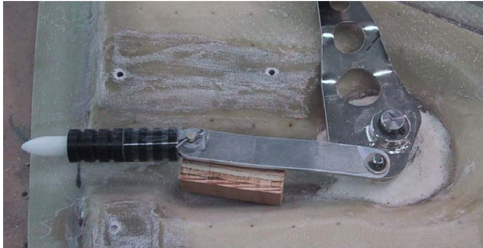
Figure 138.5: Latch Guide Sleeve Shown Ready for Bonding.
