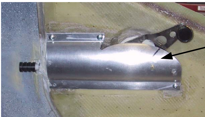
Figure 139.1: Installation of the Latch Cover Plate
