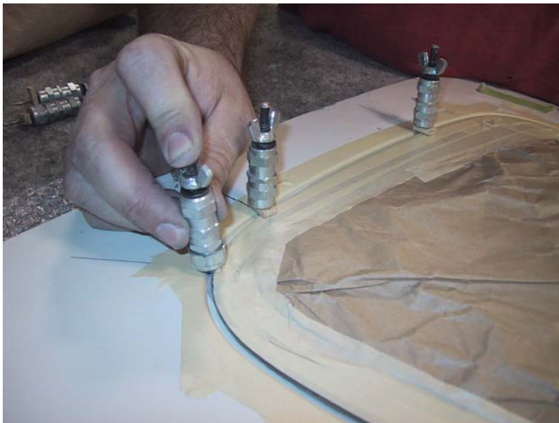
Figure B: Installation procedure for the wingnut Clecos
