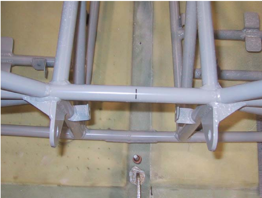
Figure 14.1 Marking the centerline on the firewall
