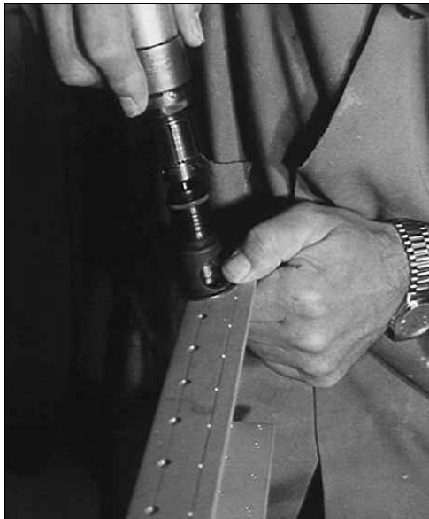
Figure 48: Countersinking the Spar
