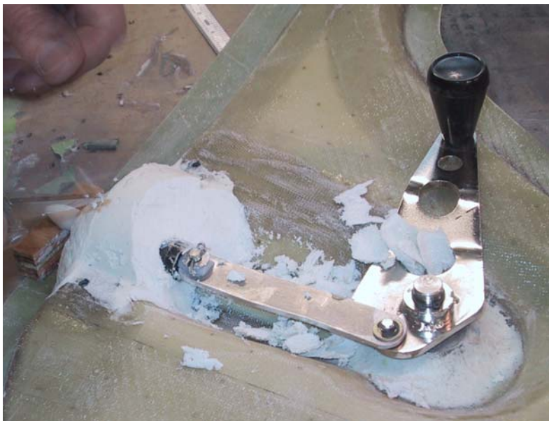
Figure 139: Bonding in the Guide Bushing
