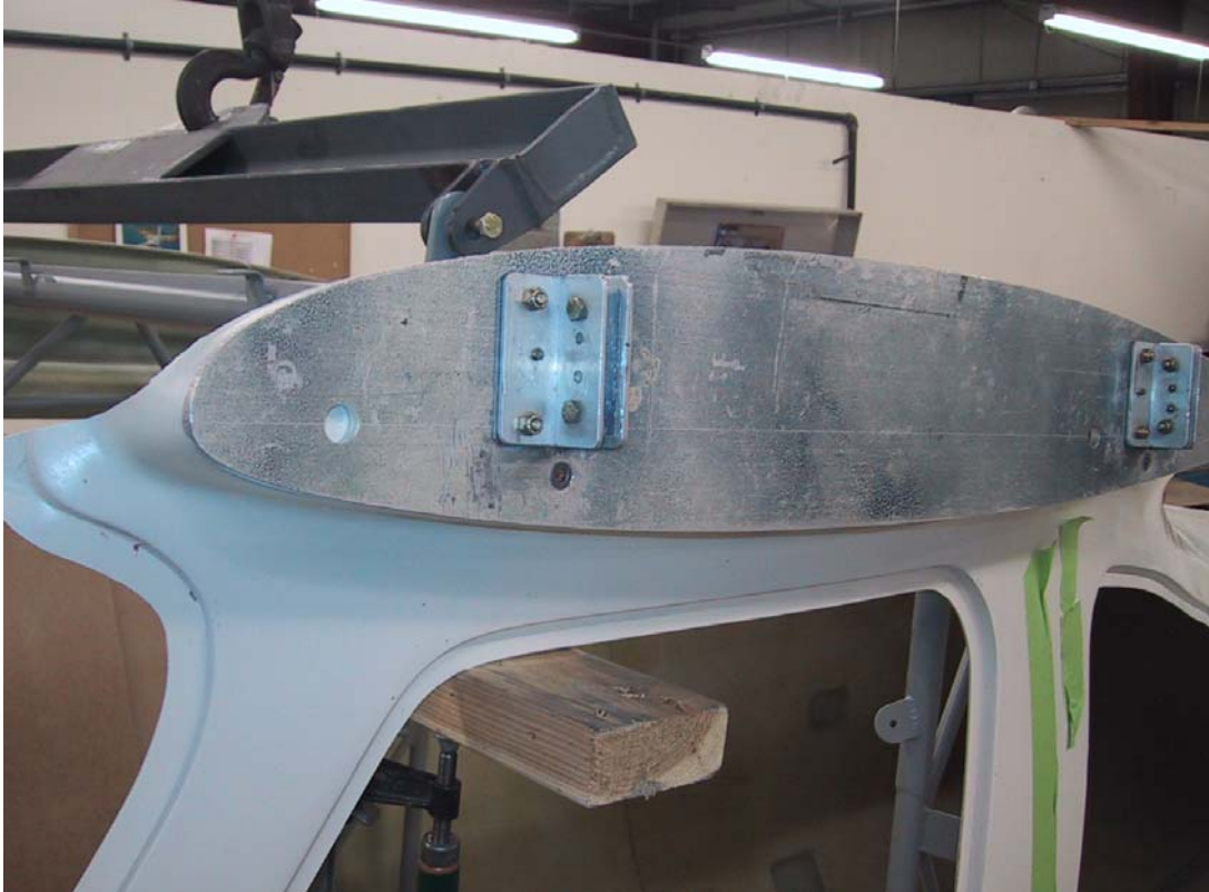
Figure 16: Wing root jigs mounted on the fuselage
