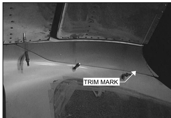
Figure 146: Fitting the Lower Hatch Cover Trailing Edge
