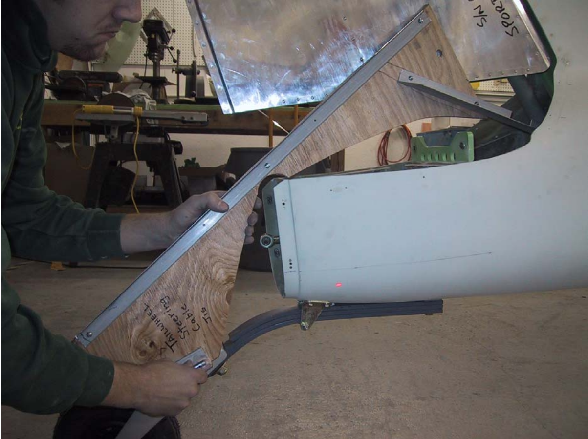
Figure A: Laser Jig for Locating the Tail Wheel Steering Cable
