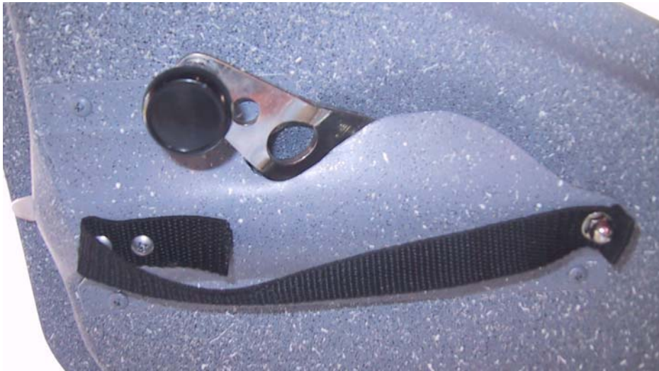
Figure 140: Final Installation of the Latch Cover Plate and Handle Strap
