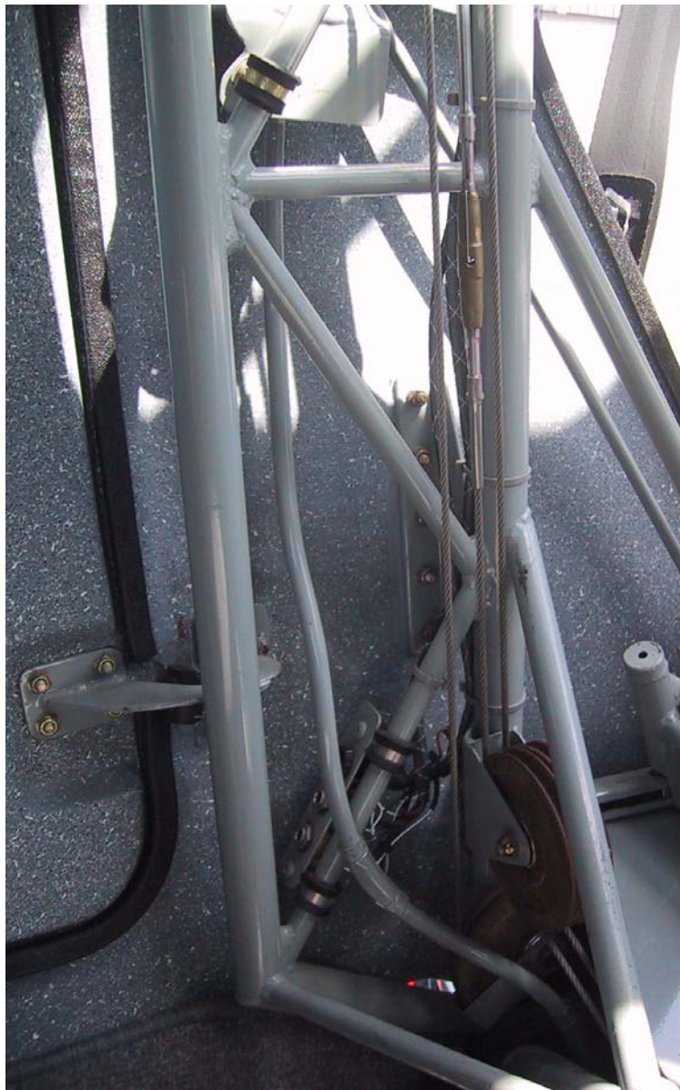
Figure 165: Routing the Fuel Line Below the Header Tank
