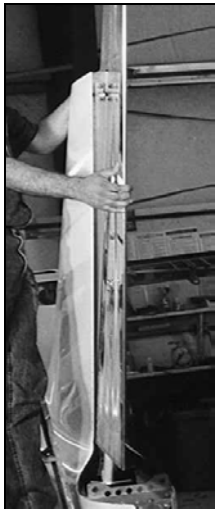
Figure 68: Hanging the Rudder
