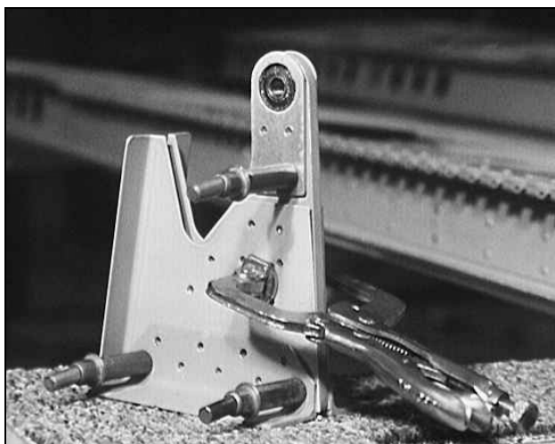
Figure 50: Assembling the Aileron Hinge
