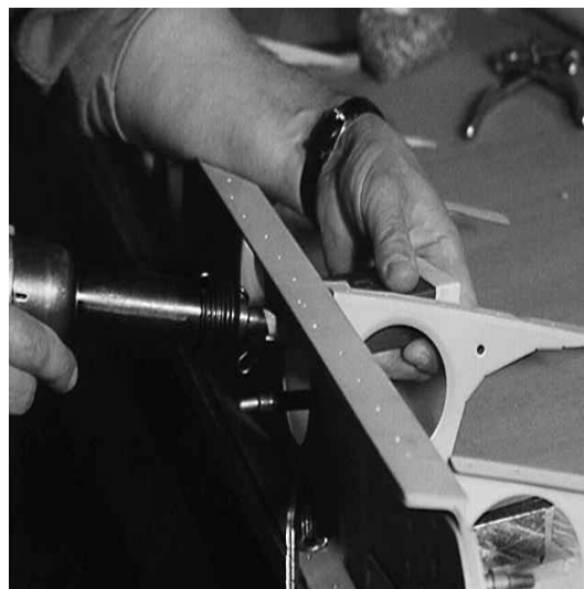
Figure 80: Riveting the Flap Cove Ribs
